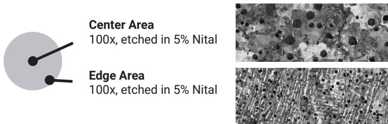
The microstructure consists of Type I & Type II nodular graphite as defined in ASTM A247. The matrix is highly pearlite with small amounts of ferrite. The edge or rim will have a higher nodule count and contain slightly higher ferrite concentration when compared to the center. Chill carbides will be less than 5% in any field at 100x and will be well dispersed.
