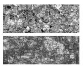
The microstructure will contain Type VII, A, size 4-6 graphite as defined in ASTM A247. The matrix is fully pearlitic. The edge or rim will consist of Type D, size 4-6 graphite in a matrix consisting of 80% pearlite. Chill carbides will be less than 5% in any field at 100x and are well dispersed.
