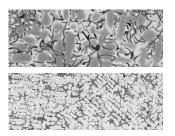
The microstructure will consist of Type VII, A, size 4-6 graphite as defined in ASTM A247. The matrix will be austenite with 5-10% alloy carbide. The edge or rim will contain Type D graphite, size 6-8. Chill carbides are less than 5% in any field at 100x and will be well dispersed.
